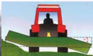
The wings float up to 25° above and below the cutting plane
