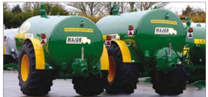
2150 Alpine tank compared to a standard 2400LGP 14" drop at the rear and 6" drop at the front
