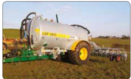
MAJOR 2600LGP with a 6.4m trailing shoe injector
